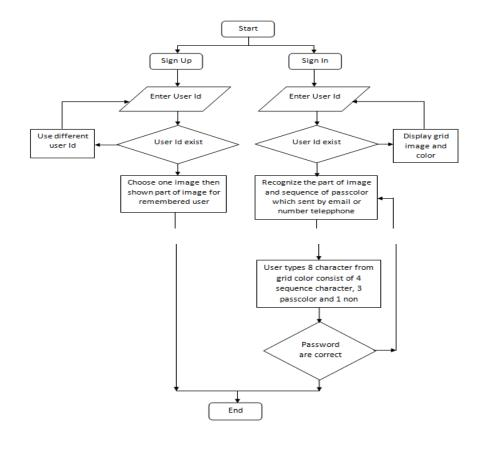
Fig 2. Flowchart of Registration and Aunthentication
