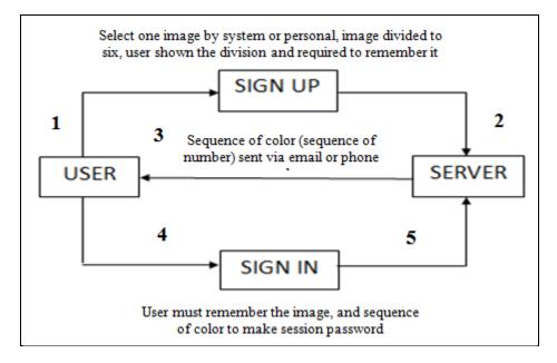
Fig 1. Architecture of Registration and Authentication
