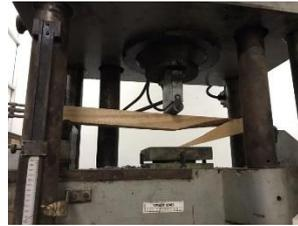
Figure 4. Mechanical bending of wood in the laboratory
