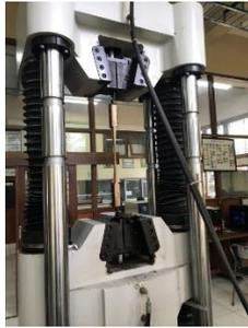
Figure 2. Mechanical testing of tensile wood parallel to fibers in the laboratory
