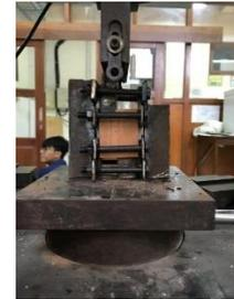
Figure 5. Mechanical shear testing in the laboratory
