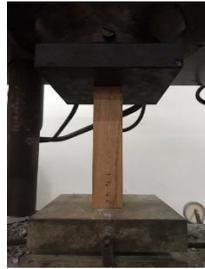
Figure 3. Mechanical testing of wood press parallel to fibers in the laboratory
