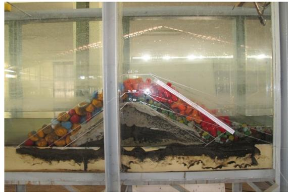
Fig. 5 Side view of rubble mound breakwater model with slope 1:1.5
