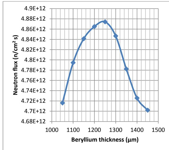
Fig. 4 Neutron flux vs beryllium thickness graph
