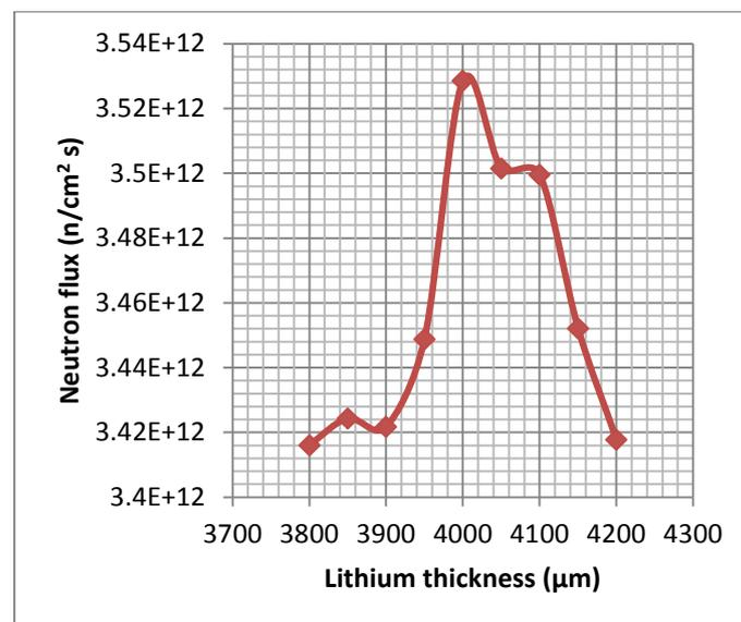
Fig. 5 Neutron flux vs lithium thickness graph
