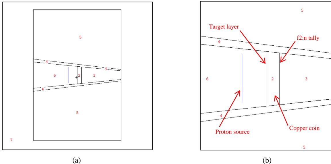
Fig. 2 (a) BSA front collimator and target geometry (b) Target geometry in details
