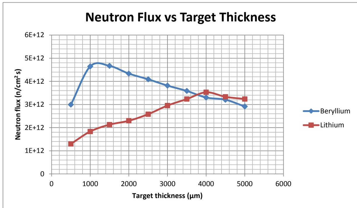
Fig. 3 Neutron flux vs target thickness graph
