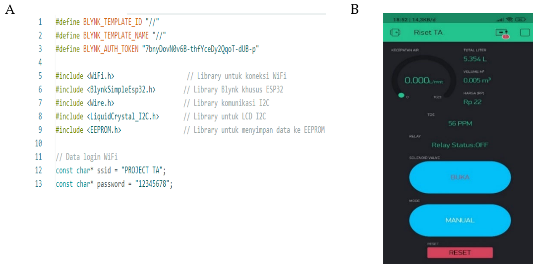
Gambar 7. a) Program ESP32 IoT, b) Tampilan Blynk IoT
