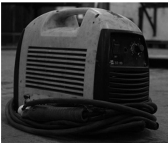
Figure 8. Arch Welding Inverter
