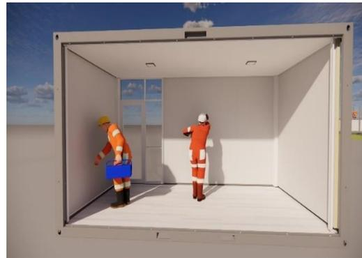
**Gambar 7. Pemasangan Dinding Sandwich Panel**
