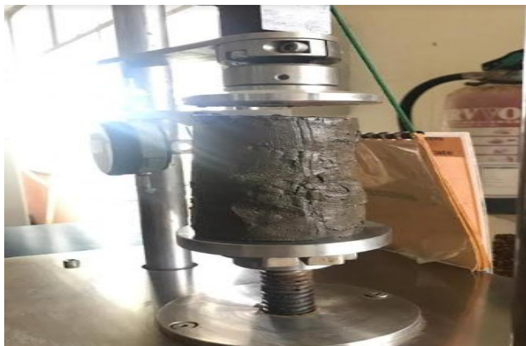
Gambar 4. Model uji UCT hasil temperatur 200 0 C
