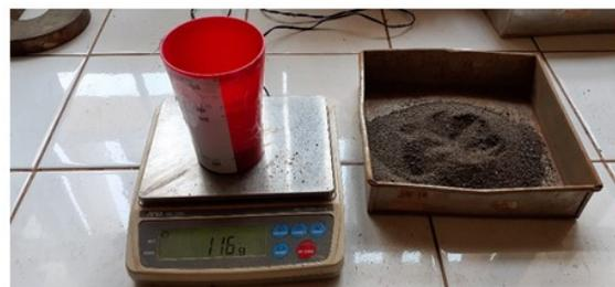
**Gambar 5.** Penimbangan material (bahan campuran beton)
