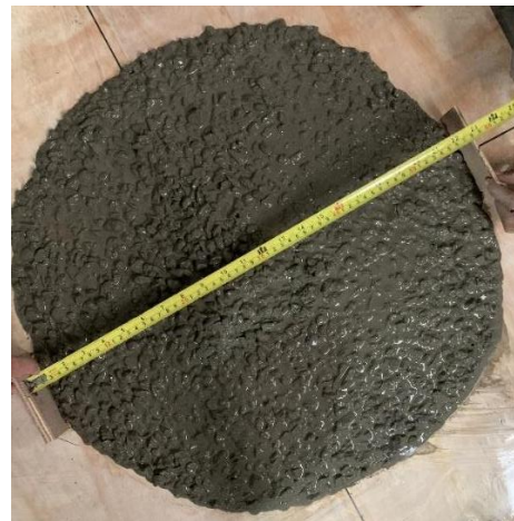
Gambar 5. Pengujian slump flow
